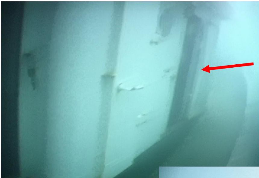
Fig. 10 (port): picture of the sunk Tugboat. The starboard watertight door (red arrow) provided access to the engine room through a staircase was found in open position.
