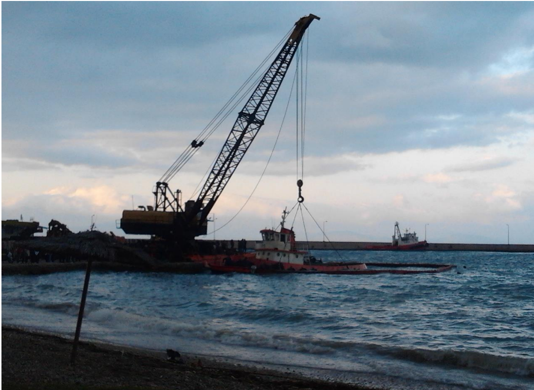
Figure 5: Refloating of T/B ARTEMIS V in Kiato Port, by a heavy lift barge.
