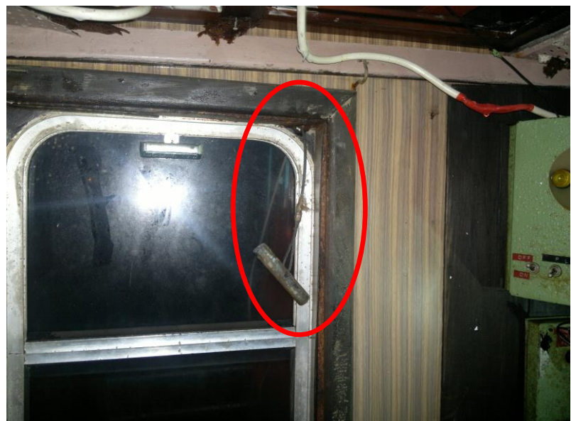
Fig. 9: The quick release activation handle inside the bridge of ARTEMIS V.
